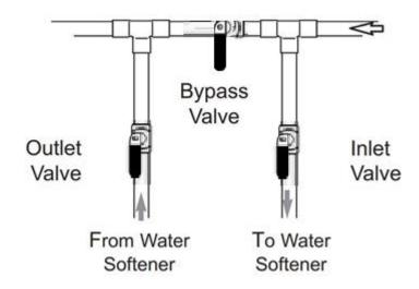
Turn off inlet valve by turning it perpendicular to or across the pipe.
